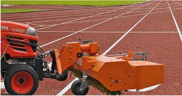
Basic cleaning can be carried out using a sweeper
